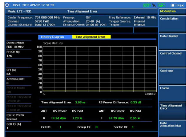
Modulation analysis — Time Alignment Error
