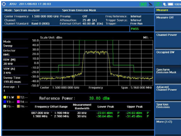
RF test — Spectrum Emissions Mask
