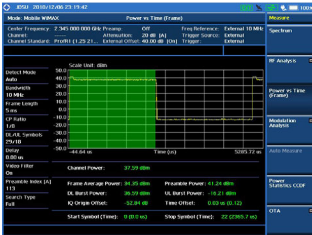
Modulation analysis — Power vs. Time
