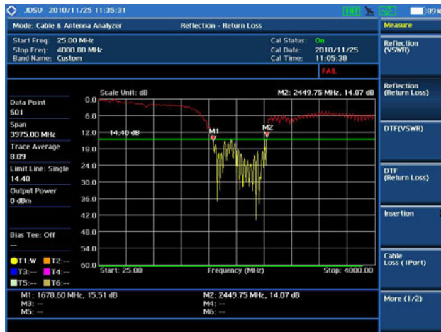
Cable and antenna test — Return Loss
