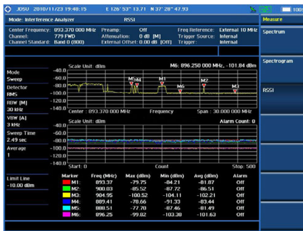
Interference analysis test — RSSI
