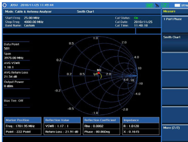
Cable and antenna test — Smith Chart
