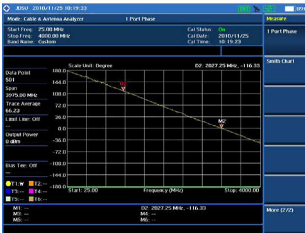
Cable and antenna test — 1-Port Phase
