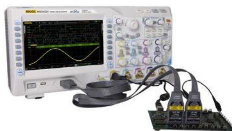
Figure 10 To Connect the Logic Probe
