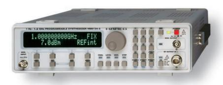
Option H085, high- stability oscillator with a stability of  $\pm 5 \times 10^{-9}$  per day
