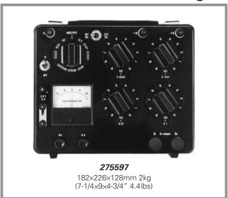
Model 2755 measures resistances from  $1\Omega$  to  $10~M\Omega$  by operation of dials and switches. Batteries and a galvanometer are self-contained. The front control panel is provided with power and galvanometer circuit selectors, one ratio arm dia, and four measuring arm dials.
