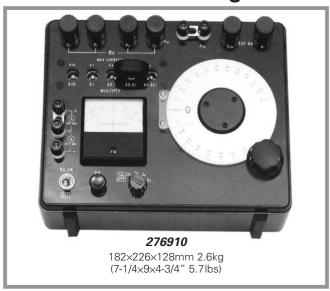
Model 2769 is a compact, portable Kelvin double bridge designed for measuring low resistance from 0.1 m $\Omega$  to 110  $\Omega$  with four multiplication plugs and one measuring dial. It has built-in standard resistors, bridge power source and high-sensitivity taut-band suspension system electronic DC galvanometer.
